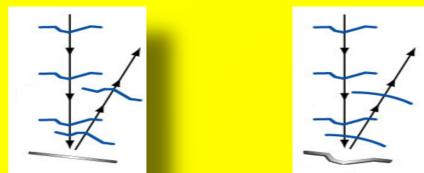
The servo control computer must make corrections faster than the seeing can change (~1 kHz). The NST AO-308 system makes these corrections at about 1.9 kHz (1,900 times per second).
