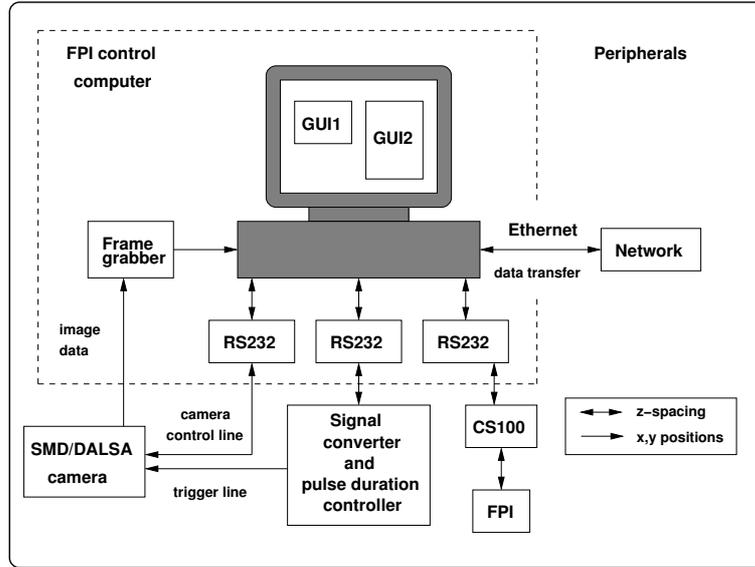
Figure 1. Schematic control and acquisition structure of the instrument.
